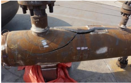
Brittle Failure / Low Temperature
