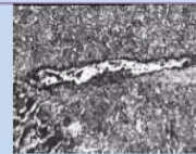
Thermal fatigue alloy steel 100X
