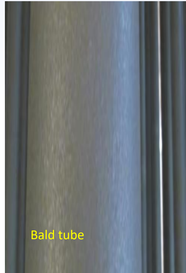
Comparison between two reformer tubes for showing baldness
