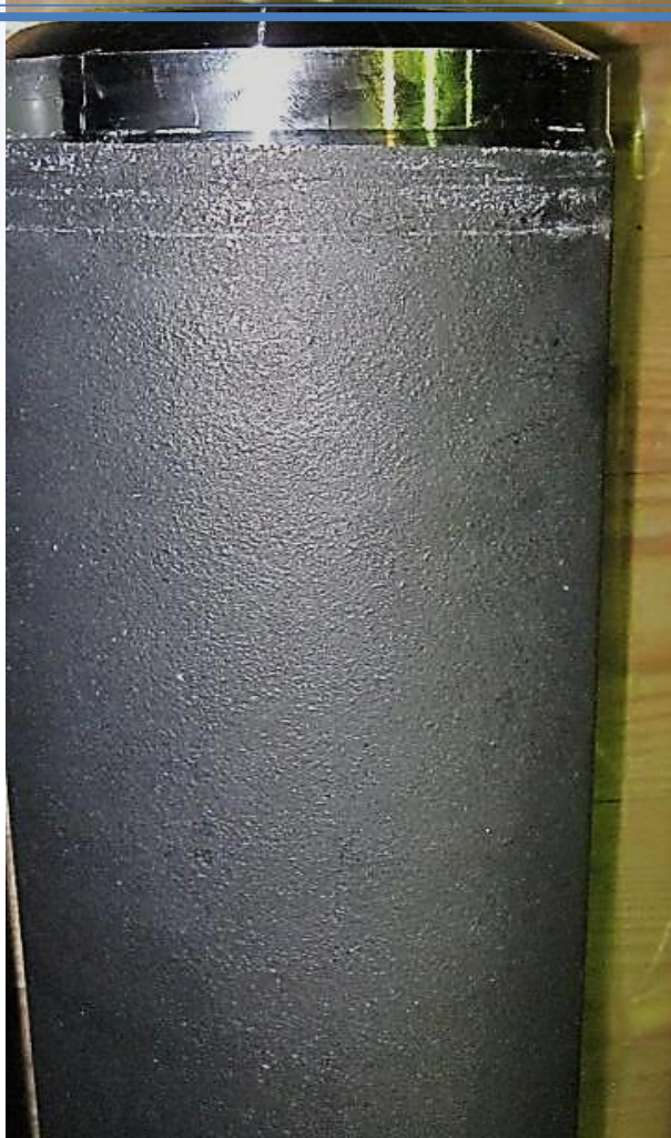
Comparison between two reformer tubes for showing baldness
