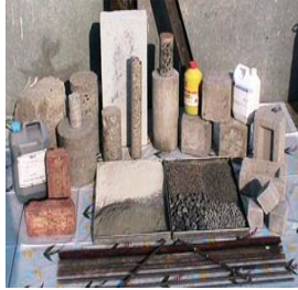
Concrete cored and sampled specimens
