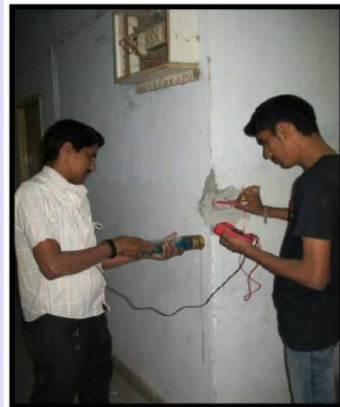
Half cell potential test
