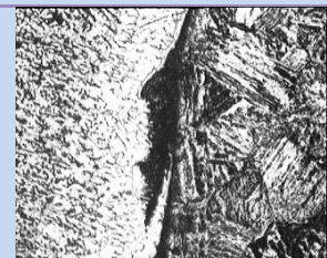
Dissimilar metal weld SS-alloy steel 200X
