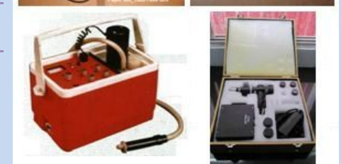
In-situ Metallography by replication method.
